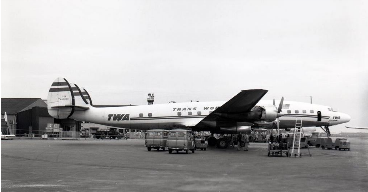
N8083H – “Eight-Three-Hotel” – seen at London-Heathrow in the late 1950s. Although the long nose could accommodate it, the ex-LAI Starliners flew without radar in passenger service. (Peter Keating photo)
