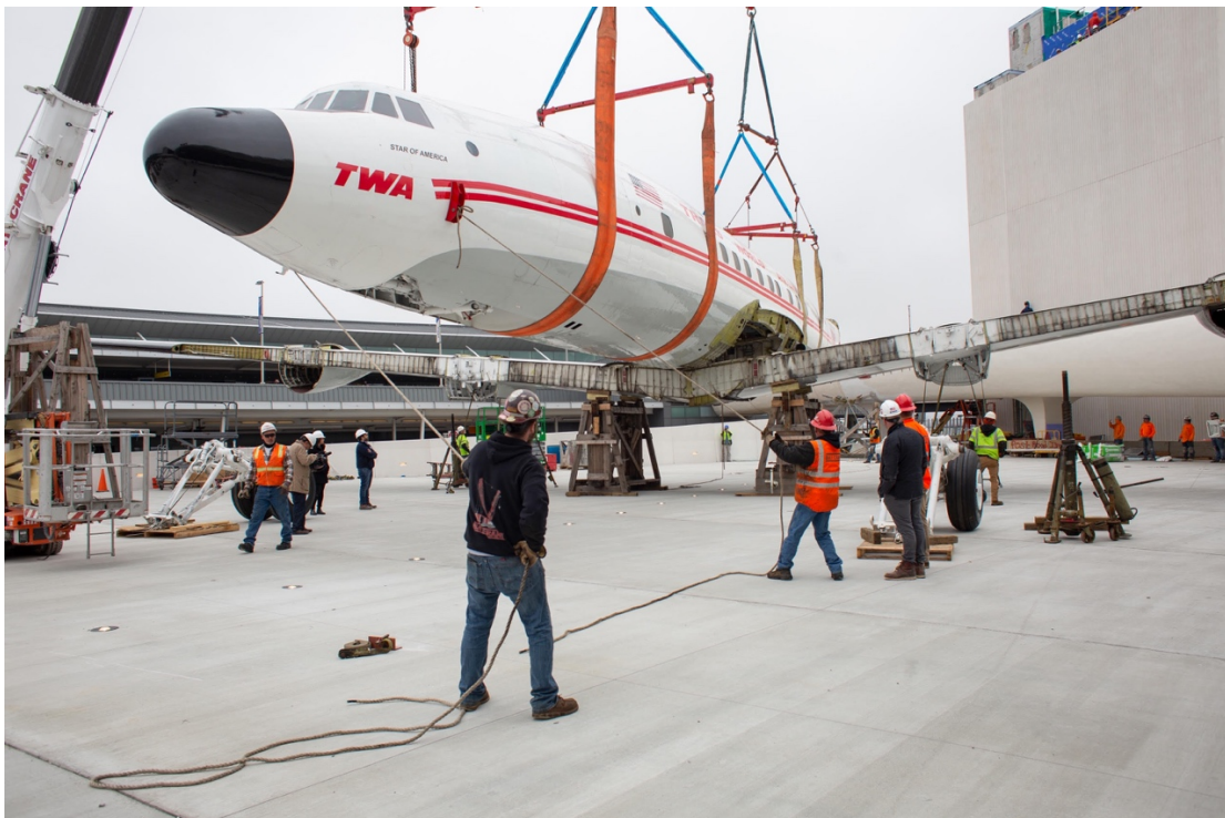
Workers gently attach Eight-Three-Hotel's fuselage to its wings. (MCR photo)
